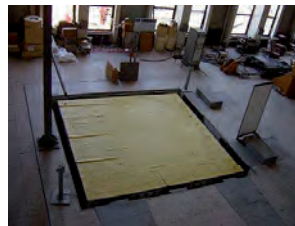
Figure 1. The shaking table in IZiIS
