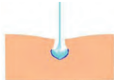
Figure 6 Penetration of the water jet and deformation of the sand after 0.03s
