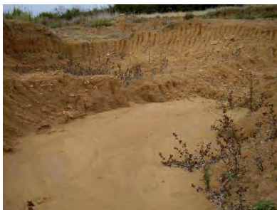
Picture 2. Example of suffosive acting of ground water on the location
