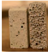
Figure 8. Two different types of foam glass aggregate prisms left fine pores, right coarse pores.
