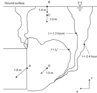
Figure 4. Contour of the plastic zone and displacement vectors (not scaled) of points A, B, C and D at t=t_c=2.4 h (ultimate state).
