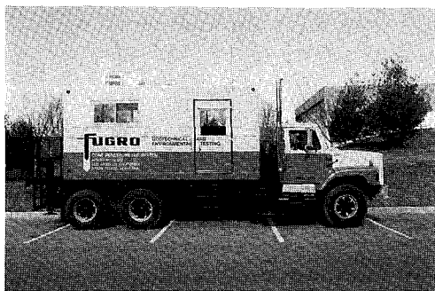
Fig. 2. Cone operated by Fugro Geosciences; manufactured by Hogentogler & Company.
