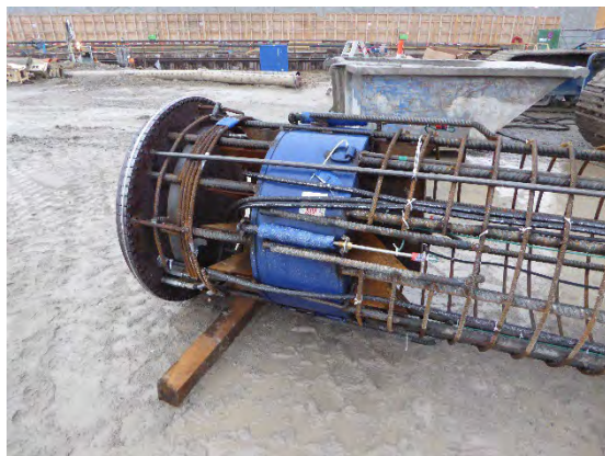
Figure 223: Flat-jack and O-cell mounted on reinforcement cage.
