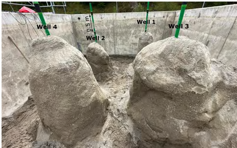
Figure 31, Sand columns obtained as a result of the MICP treatment applied in the upscaling experiment of Büyüklü et al. (2023) [7].
