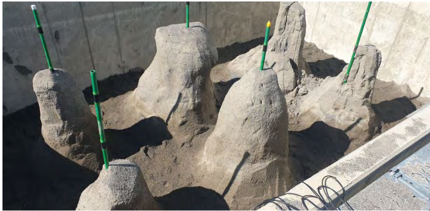
Figure 8. General view after exhuming biocemented sand columns
