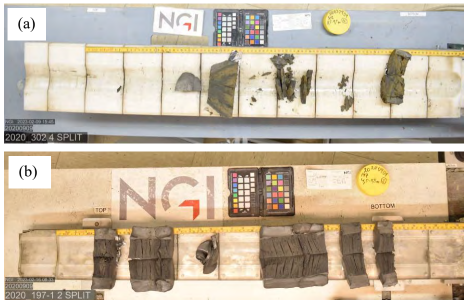
Figure 13. Piston samples. Examples of (a) dry crust intrusions, (b) laminated clay.
